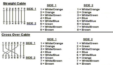
Figure A-1 Straight-Through and Crossover Cable
